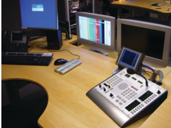
XL module, where engineer or producer can listen to and talk to 12 lines simultaneously including label transfer.
