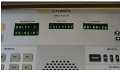
Fader start related timer, shown on producer module.
